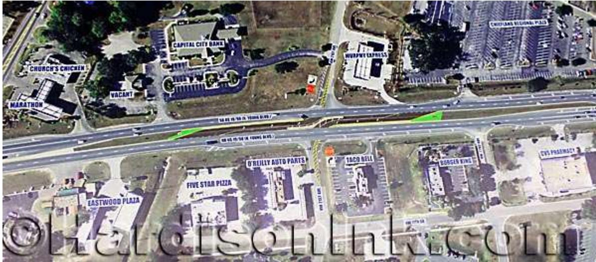
This part of an aerial photograph overlaid with graphics shows the intersection with concrete barriers, an offset for both left turn lanes off of U.S. Highway 19, some of the future signage and painting on the roads to improve safety and efficiency for motorists at this intersection. This photo is from the larger, better project display that was at the meeting on Tuesday night.
